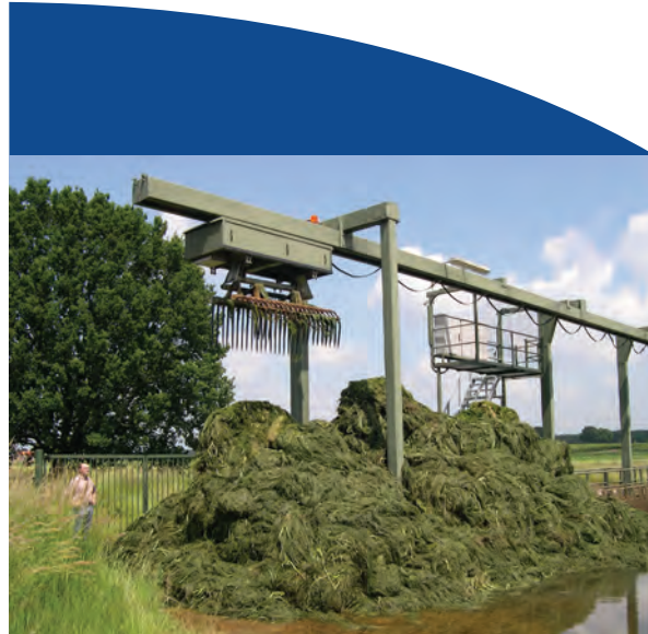
The Bosker Overhead Trashrake operating fully automatically under heavy debris conditions
